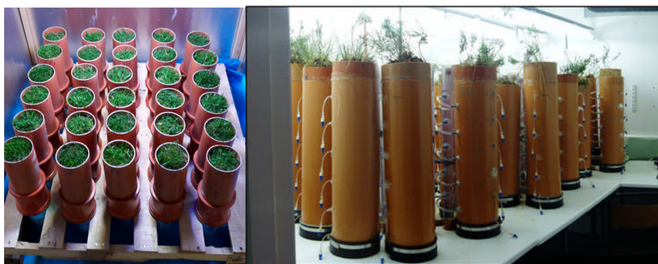
Figure 2. Left : Soil mesocosms in a controlled environmental cabinet treated with wastewater containing different concentration of pharmaceuticals. Right : Soil cores from which the soil solution can be extracted (via rhizon samplers placed at different depths) for nitrate and ammonium analysis.
