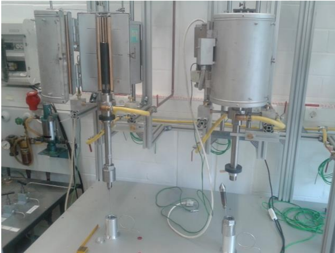
Figure 4: Cold seal apparatus with the option to perform rapid quenching to simulate abrupt changes in natural hydrothermal systems
