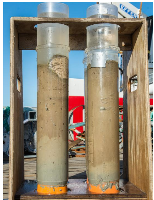
Megacorer tubes filled with ~35 cm of sediment from the Barents Sea, with brown iron-rich surface sediment and a rather unfortunate sponge in the left tube (courtesy of J Faust)
