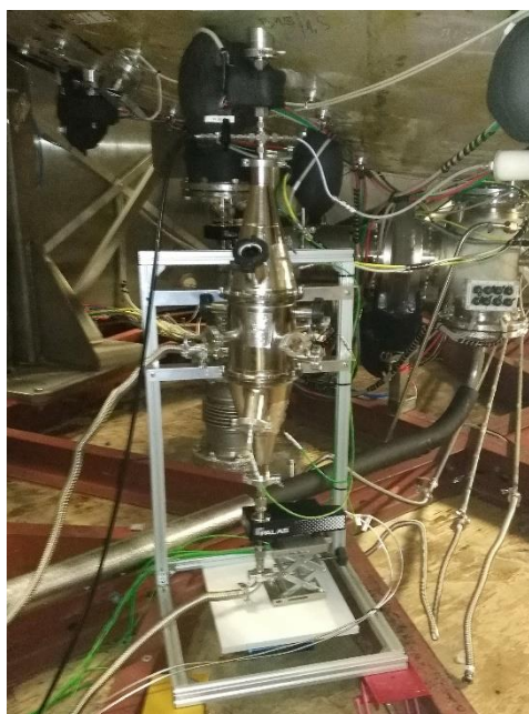
The prototype PINE chamber connected to the much larger AIDA chamber in Karlsruhe, Germany
